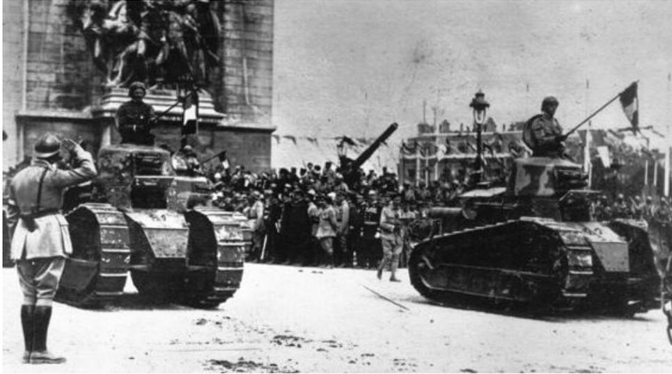
French Renault FT-17 light tanks on parade in the mid-1930s. During the First World War France helped pioneer armoured warfare with the Schneider and St Chamond assault tanks. The subsequent two-man FT-17 went into service with the French Army in 1918 and was widely exported and copied round the world. The standard production model was armed with a 37mm Puteaux gun and around 1,600 were still in use in 1940 making up half of the French tank fleet, although by then they were completely obsolete.
