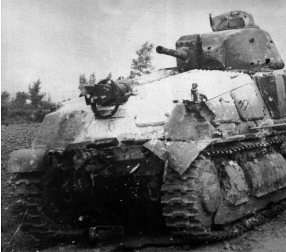
Likewise the Char Somua S-35 medium tank was well armoured with good mobility and firepower. Its turret was identical to that of the B1-bis and D2 tanks armed with the 47mm SA 35 gun and a 7.5mm Model 31 coaxial machine gun. This meant it had the usual disadvantage in that the commander had to also act as the gunner and loader during combat. About 500 had been built by the time of the German invasion.
